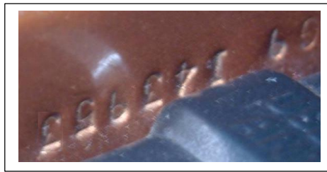
Reference top radiator core support VIN facing the radiator and stamped upside down
