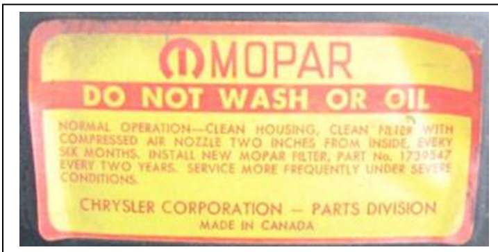
Original engine air cleaner decal - 1970 318 engine. Oct 1969 production car. Use filter part # 1739547
