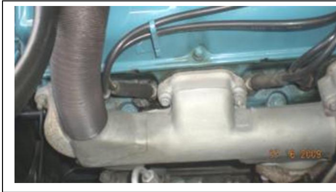
Reference 318 CID exhaust manifold with pre-air heater shield and tube.
