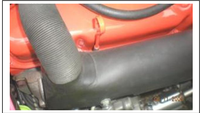
Reference 383/440 CID exhaust manifold with pre-air heater shield and tube.
