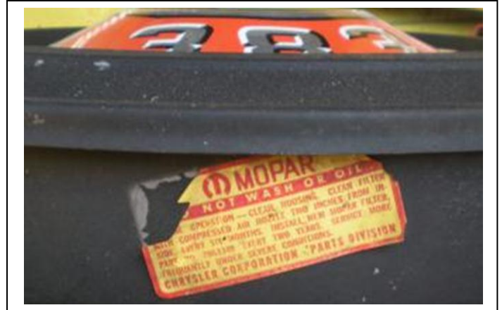
Original engine air cleaner decal - 1970 383 engine. August 1969 production car. Use filter part # 2863349. Note: The placement is on the front of the base and at an angle .
