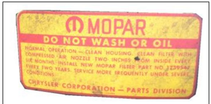
Original engine air cleaner decal - 1968 318 engine. June 1968 production car. Use filter part # 1739547 Note: the variation of Made In Canada at the bottom between this one and the one on the left.
