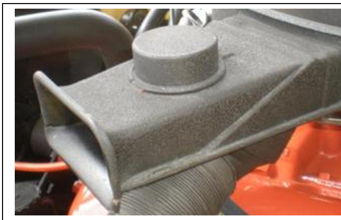
1970 reference of the vacuum diaphragm
