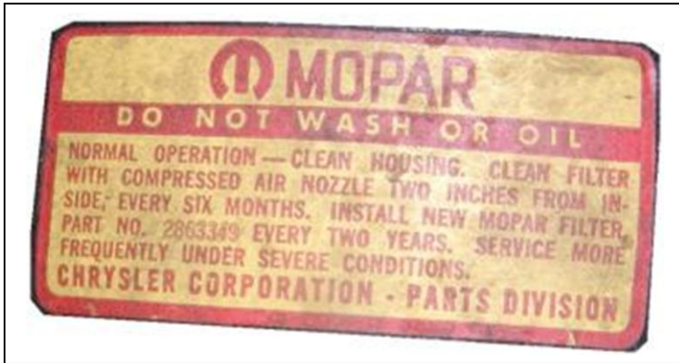
Original engine air cleaner decal - 1970 440 engine. September 1969 production car. Use filter part # 2863349
