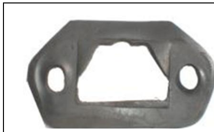
Black rubber seal between OSAC valve and air cleaner base
