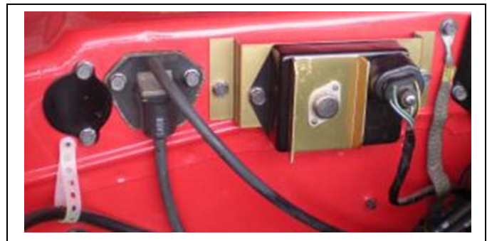
Black rubber seal between OSAC valve and air cleaner base
