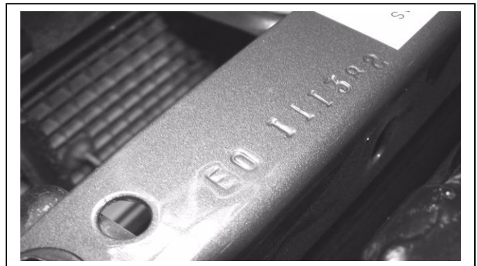
VIN on top side of core support is typically found on LA built cars
