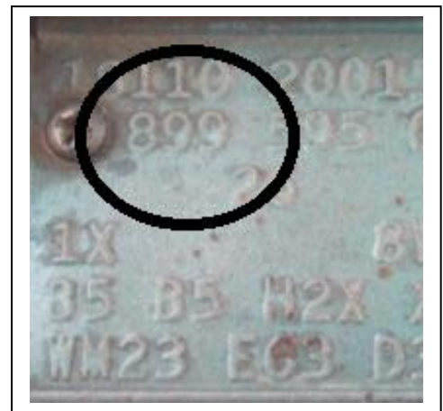
1969 Dodge Super Bee reference engine (383 4 bbl with AC) code # 899
