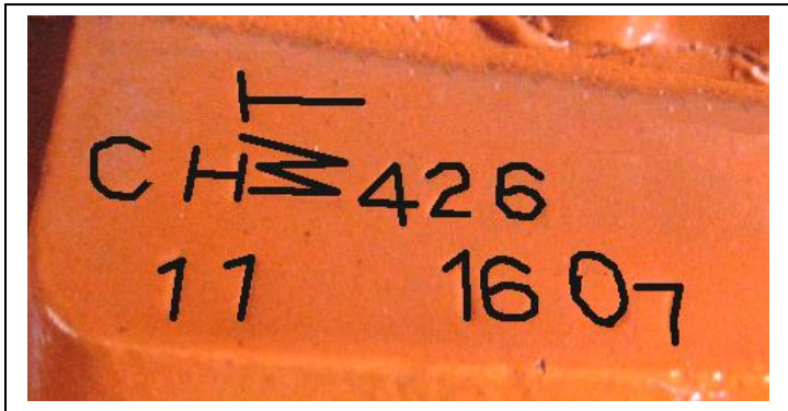
C = 1967 Production Model Year H = Hemi Engine 426 = 426 Cubic Inches WT (stamped sideways across the CH) = Water Tested Block Assembly date 11 16 = November 16, 1966 07 = 7th engine assembled that day
