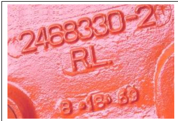
Casting # 2468330 Casting date 8 -18- 69
