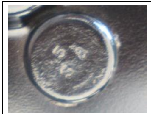
Weld nuts have been found on either side of the plate. However the majority have been found on the bottom side of the plate.
