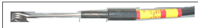
Original cables have been found with the air cleaner decal wrapped around it.
