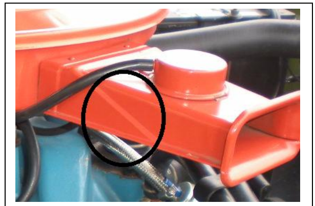
1970 383 and 440 – 4 bbl engine air cleaner early to mid model without bump
