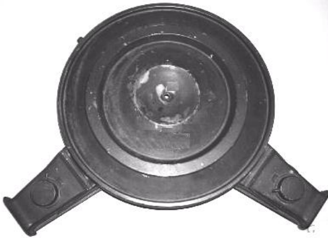
1970 383 and 440 – 4 bbl engine air cleaner early model with orange pie tin with engine call out.
