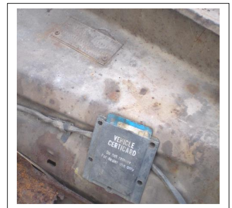
Certicard holder location on the forward area of the LH inner fender
